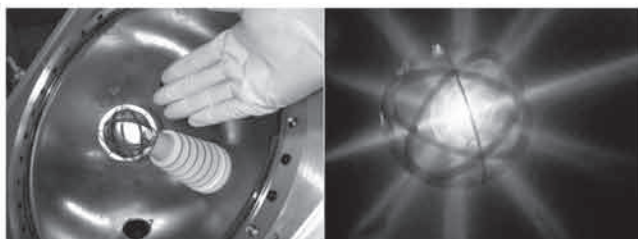
Fig. 1. The hollow cathode at the center of the spherical vacuum chamber as the anode, and an IECF plasma within the hollow cathode.
