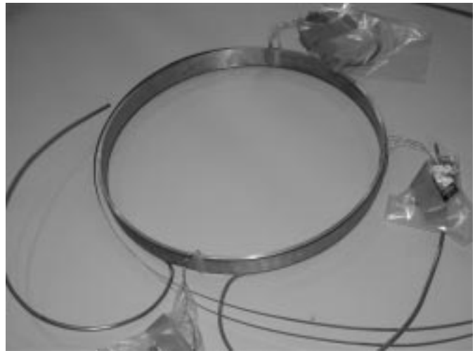
Fig. 5. Photograph of the prototype HTS-PCS developed for the Mini-RT project.
