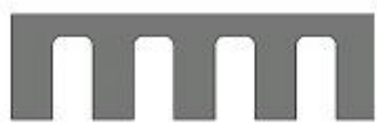
Fig 5: Rectangular micro channel with corner radius
