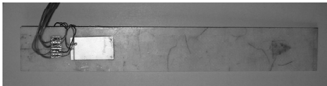
Figure 3: Composite Beam with PZT Actuator
