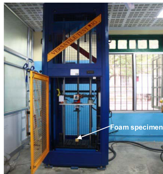
Figure 2. Impact testing machine with foam specimen placed on the base plate
