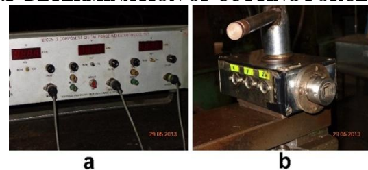
Figure 2. Electronic Dynamometer a) Digital panel b) Tool post
