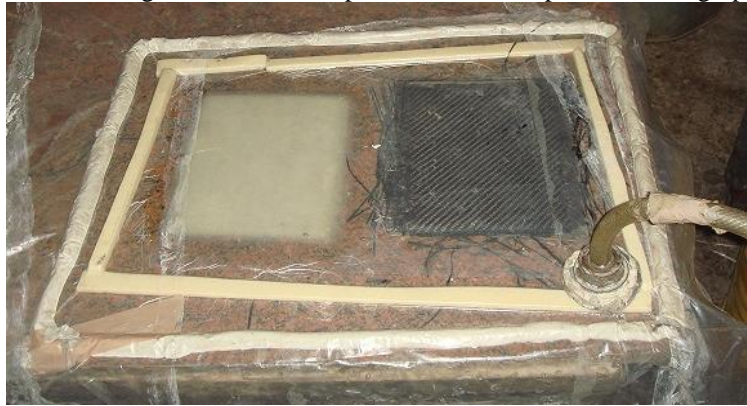
Fig – 1 Vacuum bagging Technique
