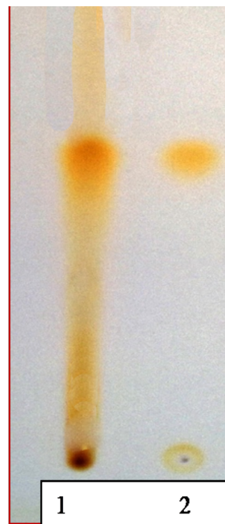
Figure 1. Detection of Lovastatin in 80:20 fraction of Benzene:Acetonitrile by TLC. Lane 1: Purified lovastatin from A. terreus (KM017963), Lane 2: Standard lovastatin
