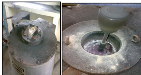
Figure. 4.4 Constituent materials are mixing. Figure. 4.5 stirring is getting done.
