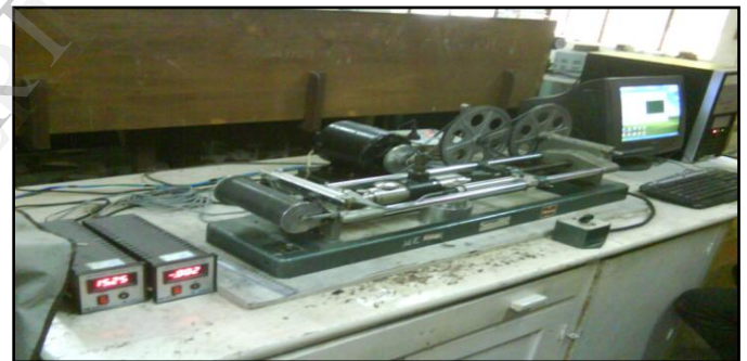
Figure 4.11: Experimental setup for Tensile Test
