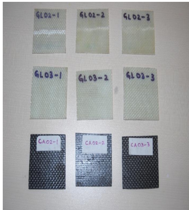
Fig 2: Damaged Specimens after Compression Test
