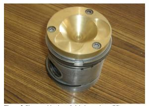
Figure 3. Photographic view of plain brass piston (BP)
