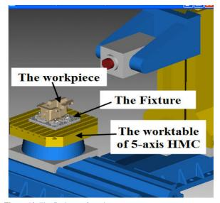
Figure 10. The final manufacturing systems
