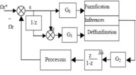
Figure 5. Fuzzy logic controller topology
