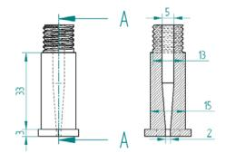
Figure 3. (b) Cross sectional view of tool
