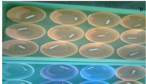
Fig. 1 Specimens dipped in NaCl Solution in 1N, 2N & 3N normality.
