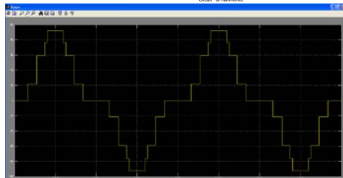
Fig. 7 Output voltage waveform result of DEA of MI=0.7
