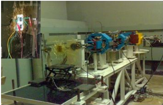
Figure 2. Experimental setup made for irradiation at Microtron Centre. (Inset shows the MOSFET placed to irradiate at bias condition)
