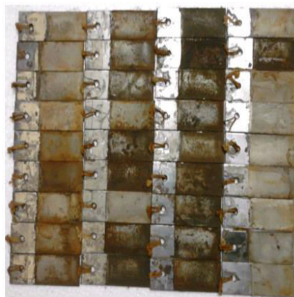
Fig 5: Ni-SiC thin coated plates after Corrosion.
