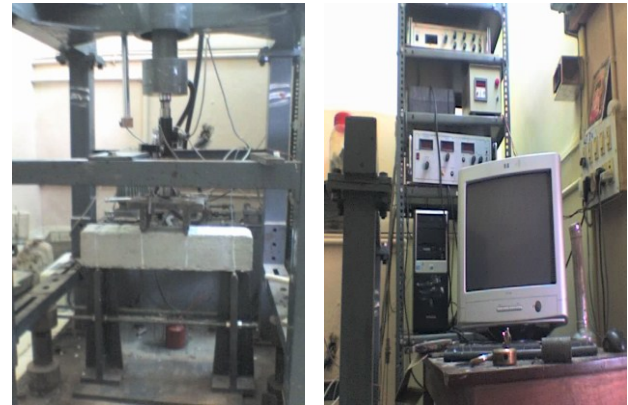
FIGURE 2 FLEXURAL FATIGUE TEST SET UP
