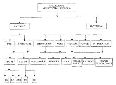
Fig. 1. Tree structure of spacecraft design.
