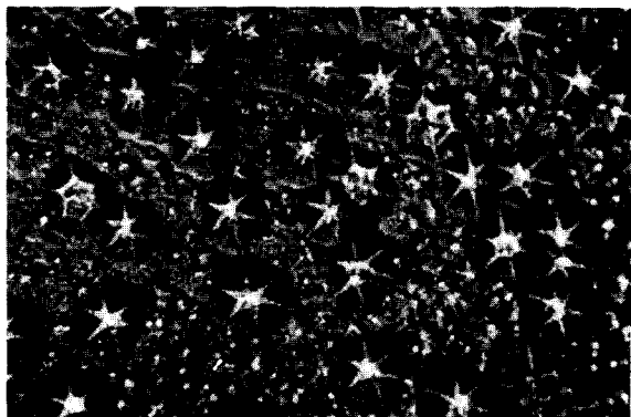
Fig. 9. Hexagonal star growth of cadmium on copper single crystals; c.d. = 20 \text{ mA/cm}^2 dc + 30 \text{ mA/cm}^2 ac.
