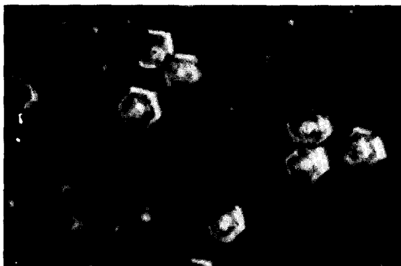
Fig. 10. Hexagonal pyramidal growth of cadmium on copper single crystals; c.d. = 20 \text{ mA/cm}^2 dc + 35 \text{ mA/cm}^2 ac.
