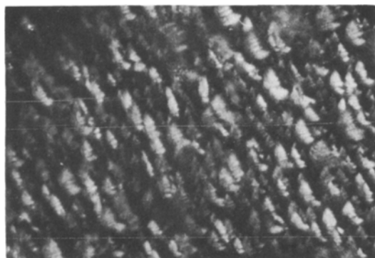
Figure 14 Dendritic growth aligned along the [110] direction on a Cu (110) plane. 0.25 M ZnSO 4 + 0.5 M (NH 4 ) 2 SO 4 bath; d.c./a.c. ratio = 15:20 mA cm -2 , × 600.
