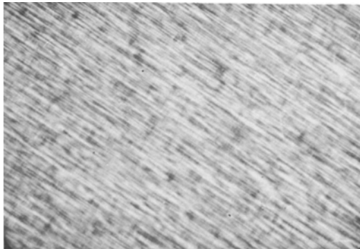
Figure 3 Ridge-type growth on a Cu (110) plane. 0.25 \text{ M ZnSO}_4 + 0.1 \text{ M (NH}_4)_2\text{SO}_4 bath; d.c. density = 10 \text{ mA cm}^{-2} , \times 600 .
