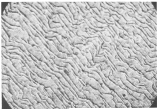
Figure 1 Layer growth of zinc observed on Cu (111) and Cu (100) planes. 0.25 \text{ M ZnSO}_4 + 0.1 \text{ M (NH}_4)_2\text{SO}_4 bath; d.c. density = 10 \text{ mA cm}^{-2} , \times 300 .
