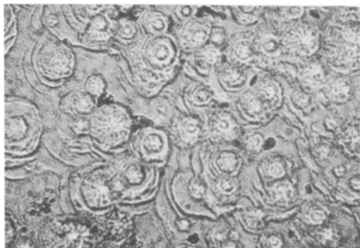
Figure 8 Distorted pyramids on a Cu (111) plane. 0.25 M \text{ZnSO}_4 + 0.1 M (\text{NH}_4)_2\text{SO}_4 bath; d.c./a.c. ratio = 10:25 \text{mA cm}^{-2} , \times 600 .
