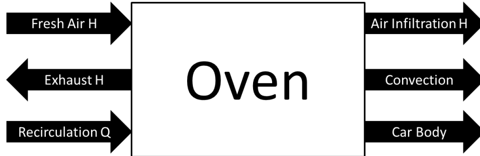
Figure 3.9 – Oven heat loss diagram
