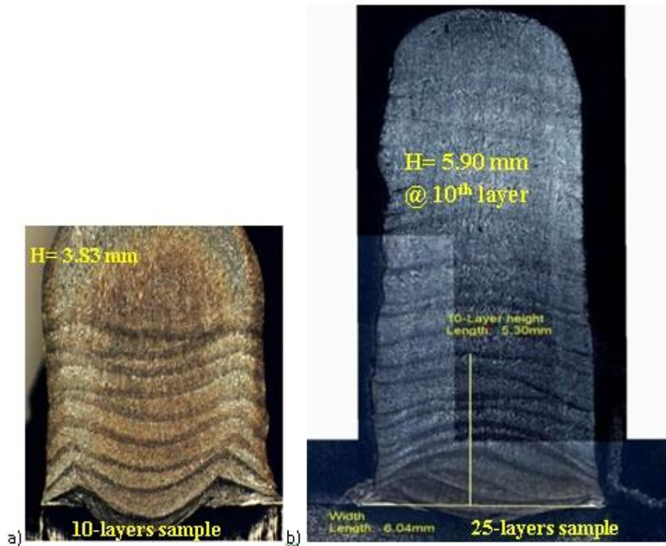
Figure 31. Comparison of heights in 10 layers and 25 layers samples
