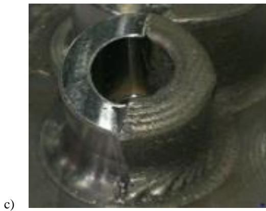
Figure 90. a) b) Models made using metal bead deposition process [128-129] c) A cladded component with half machined
