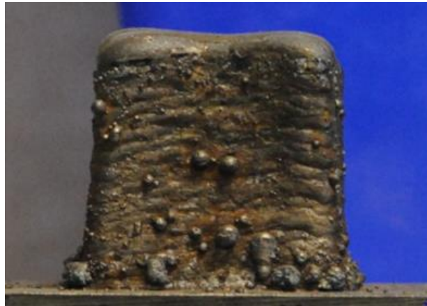
Figure 96. A cladded solid block, note the sloped corners
