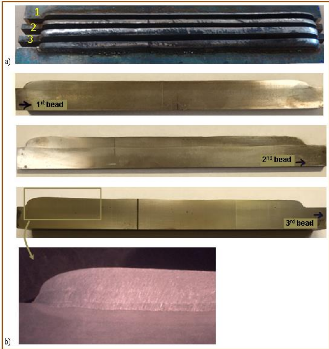
Figure 36. a) Longitudinal EDM cut of the 3x4 bead stack sample b) Cross section views of all three sections—each view contains four layers of stack--enlarged view is also shown.
