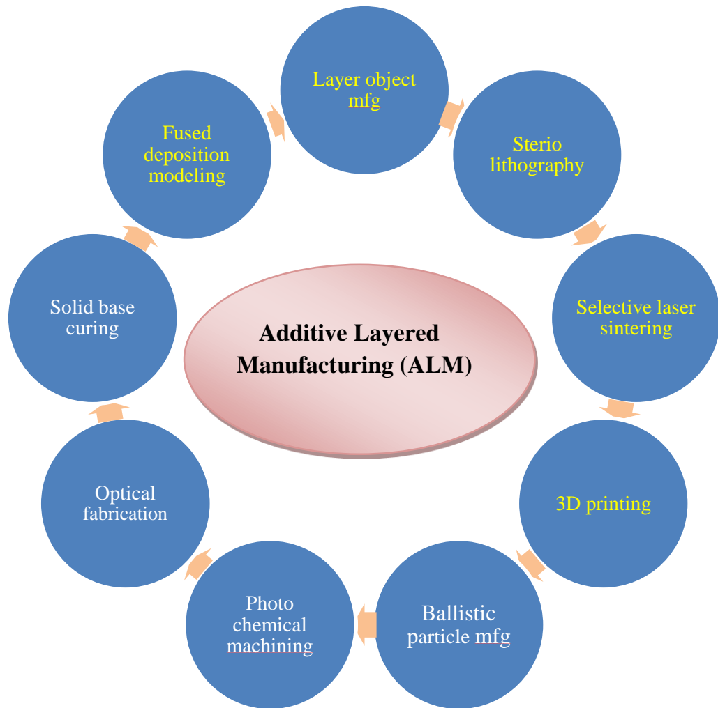
Figure 1. Different methods of additive layered manufacturing processes
