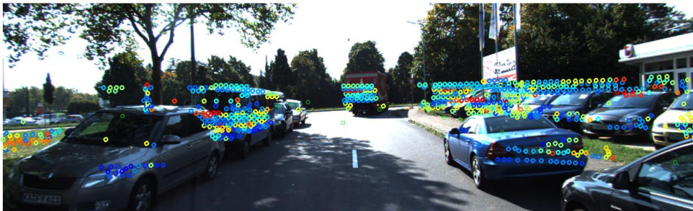
Fig. 16 Illustration of Ground plane Detection and removal from point cloud data
