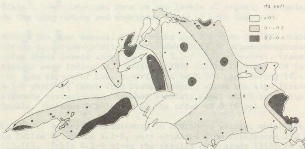
FIG. 4.1-1 The average distribution of total mercury in the surface waters of Lake Superior (1970-1971). Dots represent sampling stations.
