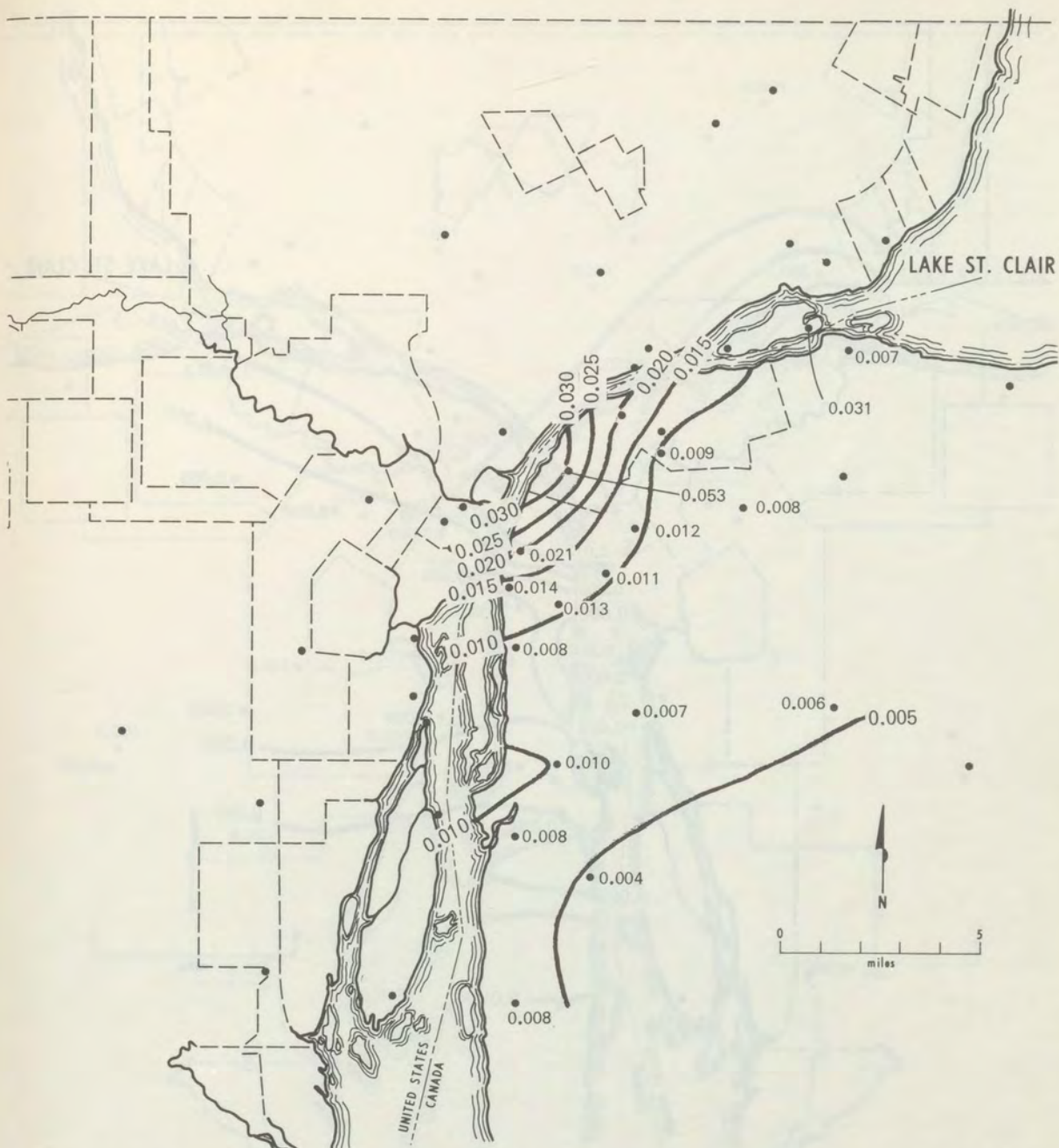
Figure 4-20. Estimated contribution of U. S. point sources to annual average concentrations of SO 2 (ppm) in the Windsor area.
