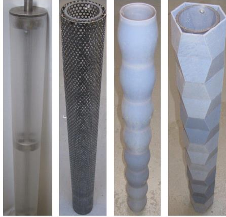
Figure 1.2 Surface modification of cables (Kleissl and Georgakis, 2011)
