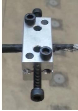
Figure 3.26 Connector used to attach cross-tie to main cable
