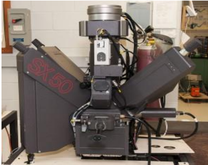
Figure 3.11: Cameca SX50 Electron Probe Micro Analyzer (EPMA) at Earth Sciences, University of Toronto [84].
