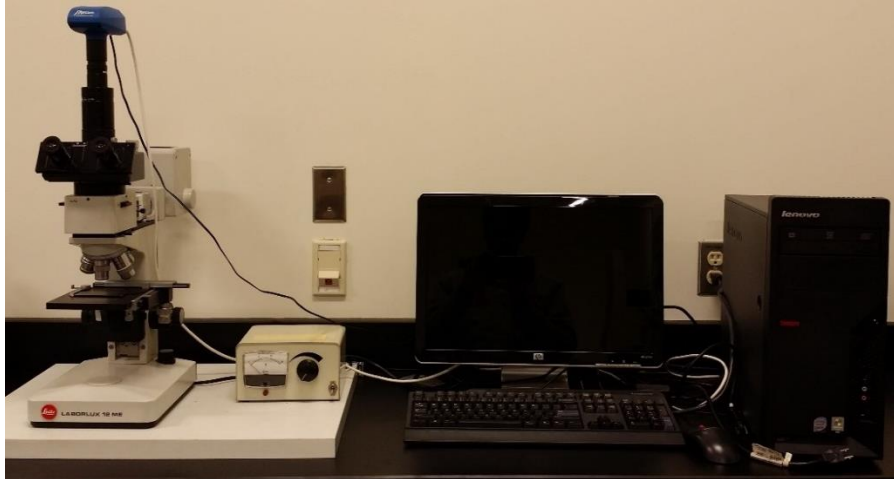
Figure 3.6: A light optical microscope (Leitz Laborlux 12 ME).
