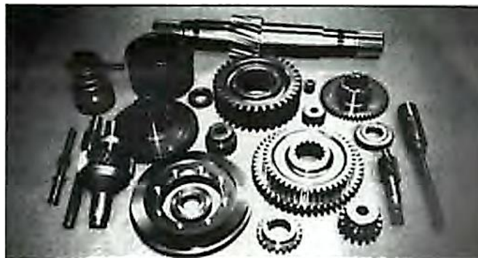
Figure 2.1: Ferritic nitrocarburized gear and other components [6].
