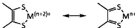
Figure 2.1 The possible resonance forms for a transition metal dithiolene complex: ene-1,2-dithiolate dianion ( left ) and neutral dithioketone ( right ).
