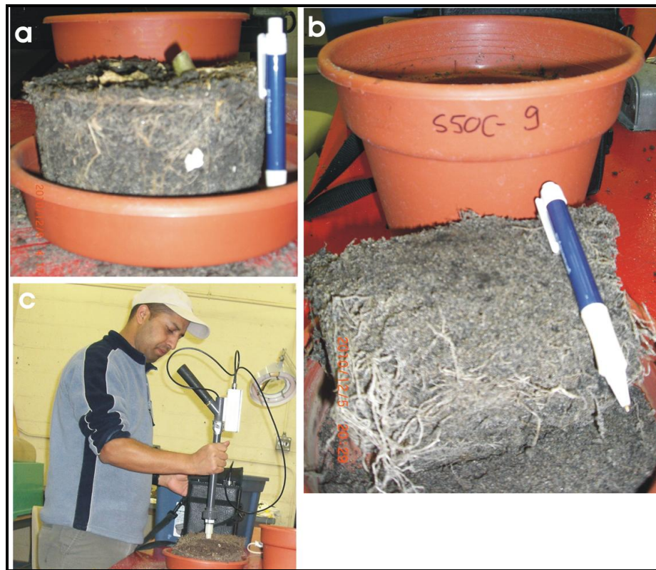
Fig. 3.2 Preparation and measurement of vertical MS profiles: (a) recovered soil from container, (b) longitudinal soil section, and (c) MS measurement along the longitudinal section using the MS2 system and a MS2F probe.
