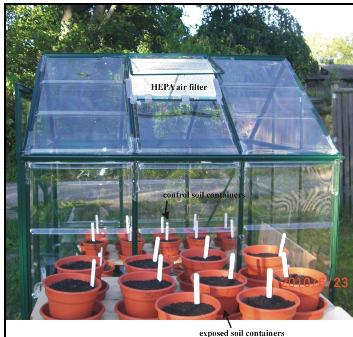
Fig.1.5 Control (inside greenhouse) and exposed (outside) soil sample sets of Experiment 2. HEPA air filters were placed in the vents to trap the majority of the atmospheric particulates while allowing air to pass through.
