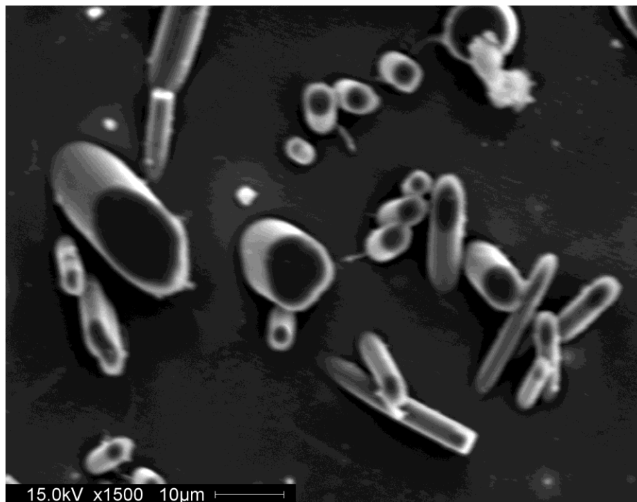
Figure 4. 9 SEM showing the interface between the fiber and the matrix for the composite with fraction of 9 vol%.
