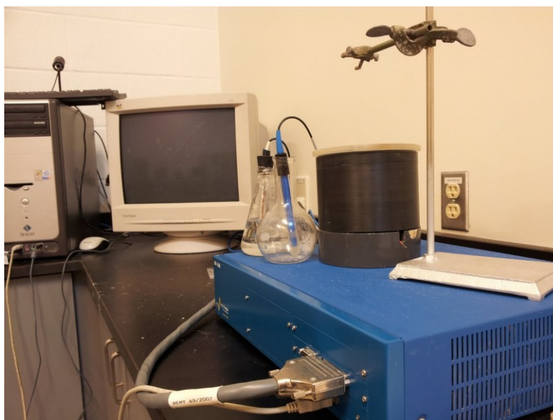
Figure 3.9 EC-LAB SP-150 electrochemical apparatus for corrosion test.
