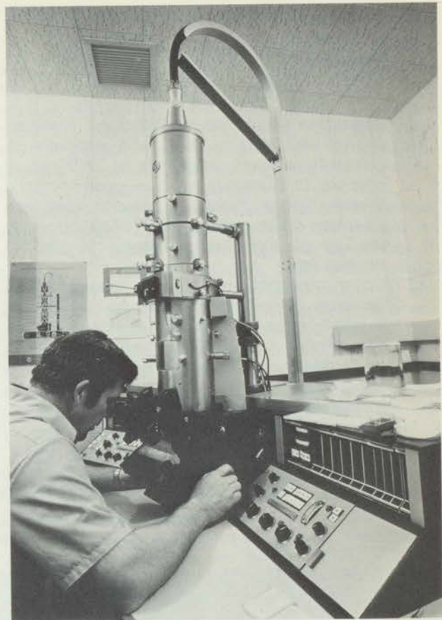
Electron microscope analysis for asbestos fibers at Duluth EPA Laboratory. (Courtesy U.S. EPA-Documerica)
