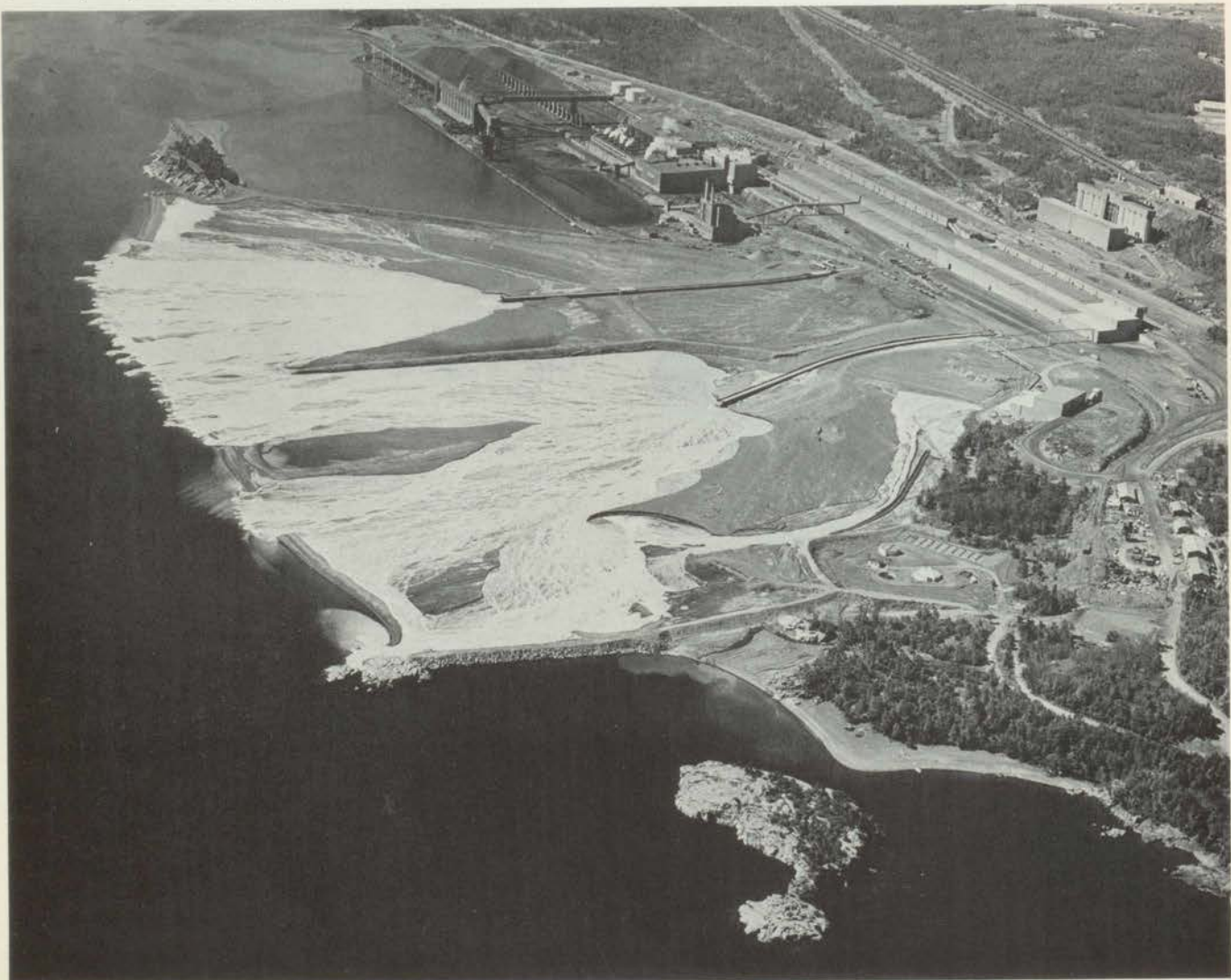
Taconite tailings discharge of Reserve Mining Company at Silver Bay, Minnesota. (Courtesy Basgen Photography, Duluth, Minnesota)
