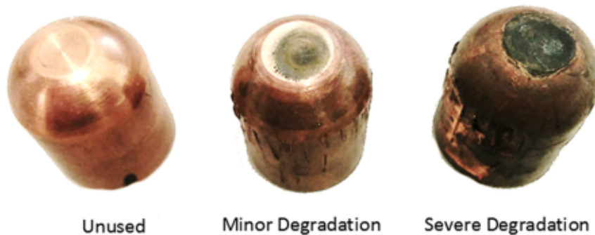
Figure 1.2 - The spot weld electrode at increasing stages of degradation, the notable surface changes in the severely degraded cap are a result of material being lost from the cap surface during welding. The rate at which caps degrade is highly dependent on the welding conditions employed.
