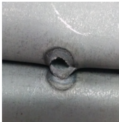
Figure 1.3 - An example of a peel test performed on a weld, the size of the welded area can be measured from the fused region after completion. Although somewhat inaccurate, peel testing is one of the fastest measurement methodologies.
