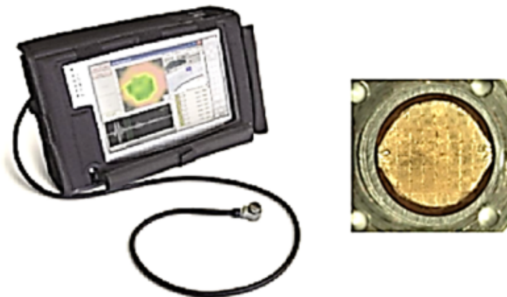
Figure 1.5 - The RSWA by Tessonics is an example of a post welding microscopy device. Using a 52 element array the size of a weld is measured using signal processing techniques (Tessonics, 2008).
