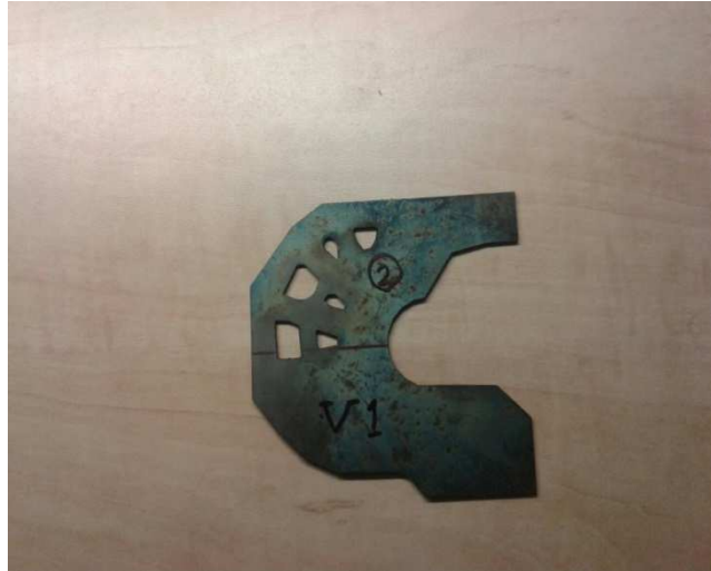
Fig 3.9 Optimized model with iso value of 0.15
