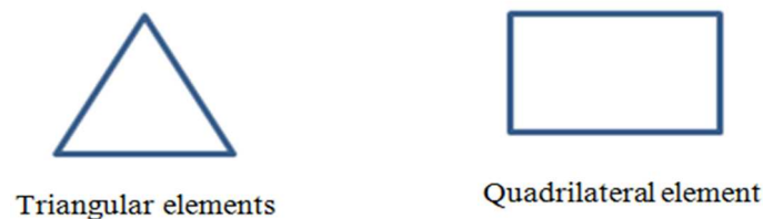
Fig 4.10 Triangular and quadrilateral elements
