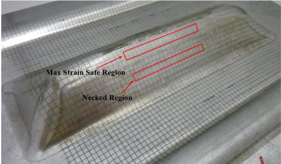
Figure 5.5. Necked and maximum safe strain regions of the DP600 EHDF specimen formed into the 38° V-shaped die using a 13 kV pulse
