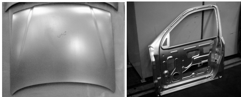
Figure 4- Pilot parts for 1st DOE project: hood outer (L) and front left door inner panels (R)
