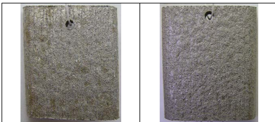
Figure 3.4: Ni-P metallization, Table 3.7, of fly-cut (Left) AM50 and (Right) AZ91D Mg alloys samples. Deposition Process: alkaline cleaning [20 min, 64 °C], acidic Mn-cocktail pre-treatment [2 min, 25 °C], Ni-P metallization [15 min, 90 °C].
