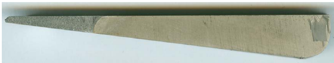
Figure 3.51: Macroscopic scanned image of a Ni-Co-P deposit [10 min, 82 °C] on a 65 mm long, 8mm wide at the base, AZ91D Mg alloy sample.
