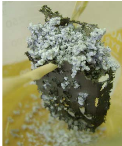
Figure 3.2: Electroless Ni-B “Hulk” coating of an AZ91D Mg alloy substrate. Deposition Process: fly cut sample, 15 min alkaline cleaning at 50 °C, 2 min acidic pre-treatment at 25 °C, 3 h metallization at 90 °C.
