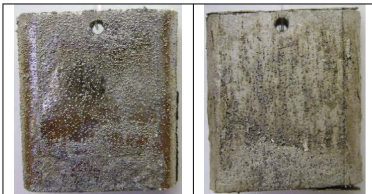
Figure 3.8: Electroless Ni-P coating on fly-cut AZ91D Mg alloys after alkaline cleaning [20 min, 68 °C], Table 3.7, and HF pre-treatment [2 min, 20 °C], Table 3.8, from (Left) HF-containing, Table 3.7, [Deposit: 7 min, 86 °C, pH 3.4], (Right) HF-free, Table 3.2, Ni-P electrolytes [Deposit: 3 min, 74 °C, pH 5.4].
