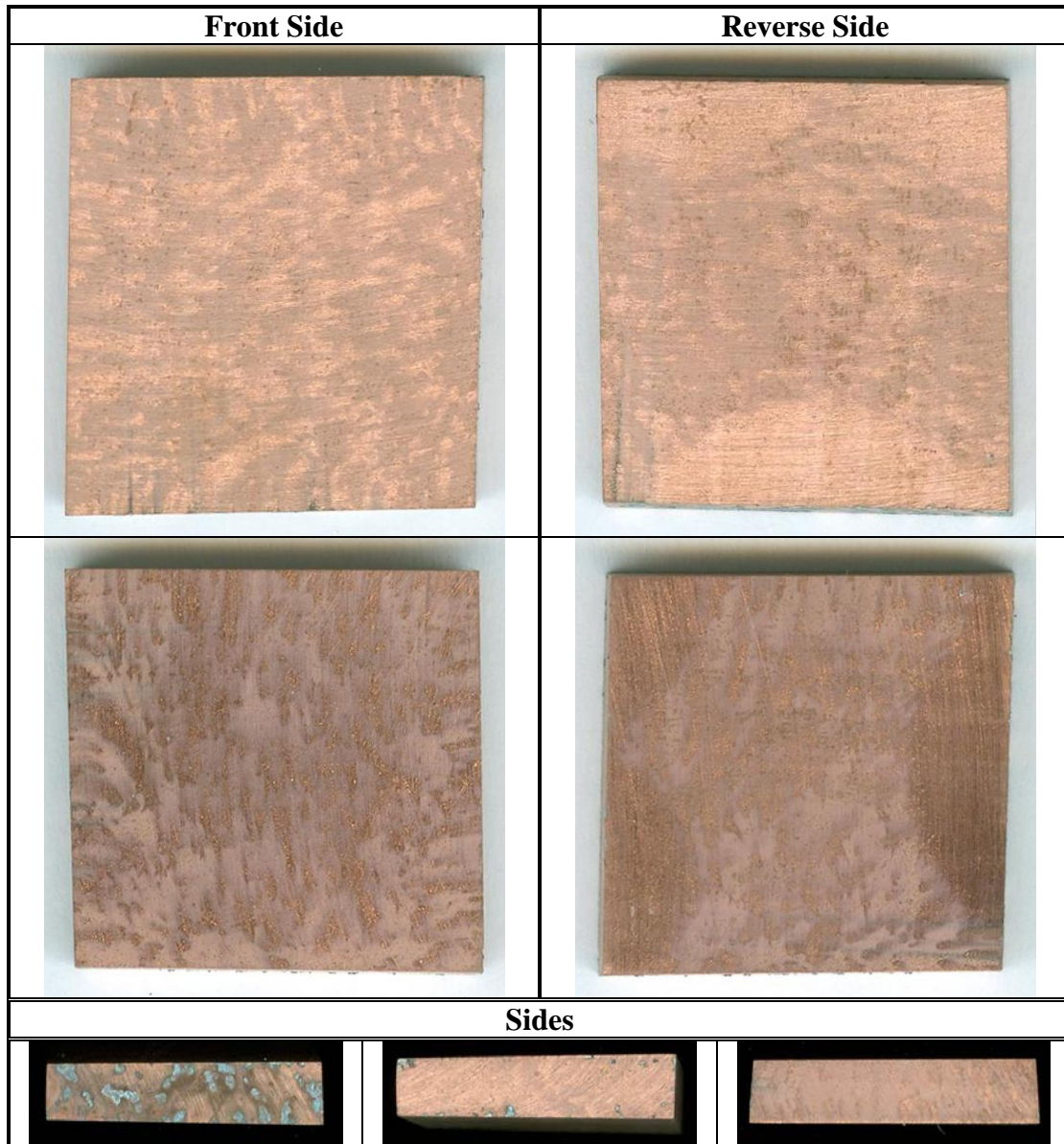
Figure 3.33: Macroscopic scanned images of an electroless Cu deposit [20 min, 25 °C] on a dry polished 25 mm × 25 mm × 5mm AZ91D Mg alloy.
