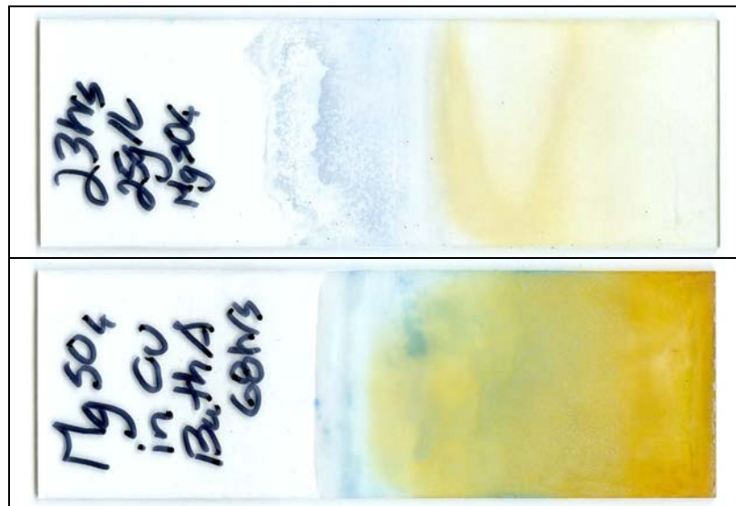
Figure 3.31: Macroscopic scans of (Top) 23 h and (Bottom) 68 h electroless immersion deposits on Sn/Pd treated glass slides, treated region 45 mm × 25 mm, from an electrolyte containing 25 g/L \text{MgSO}_4 \cdot 7\text{H}_2\text{O} , 20 g/L NaOH, 35 g/L \text{CuSO}_4 \cdot 5\text{H}_2\text{O} , and 75 g/L \text{KNaC}_4\text{H}_4\text{O}_6 \cdot 4\text{H}_2\text{O} .
