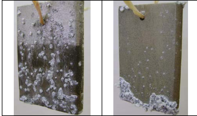
Figure 3.3: Electroless Ni-B coatings on fly-cut AZ91D Mg alloys; (Left) Deposition Process: 15 min alkaline cleaning at 50 °C, 2 min acidic pre-treatment at 25 °C, 45min metallization of the lower half of the sample at 90 °C; (Right) Deposition Process: 20min alkaline cleaning at 57 °C, 60 min stannate conversion at 90 °C, 45 min metallization of the entire sample at 85 °C
