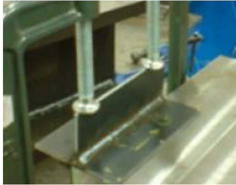
Figure 4.28- T-joint clamping condition [21]
