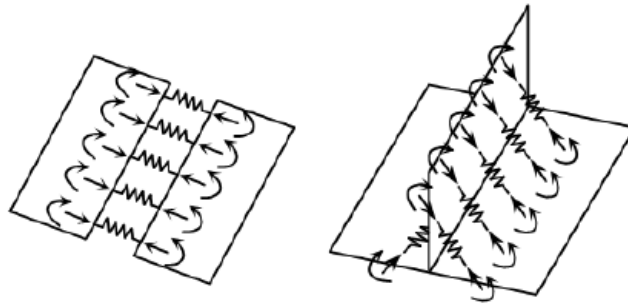
Figure 2.17-Models of shrinkage forces and moments for butt joint (left) and T-Joint (right) [21]
