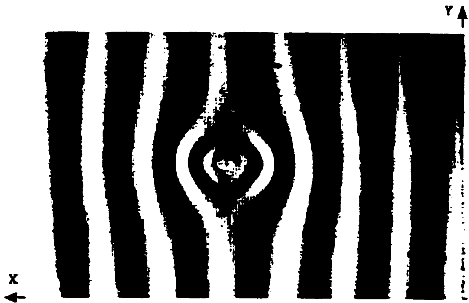
Figure 4.2a The grating image for an indent with phase shift \alpha=0
