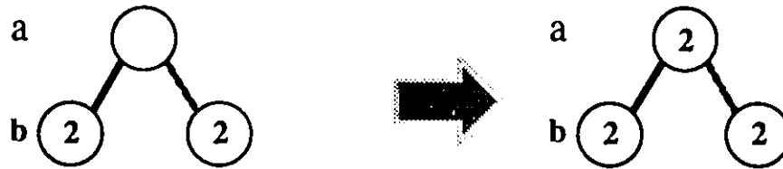
Figure 3.5 Rule 1 of Switching Tree Minimization
