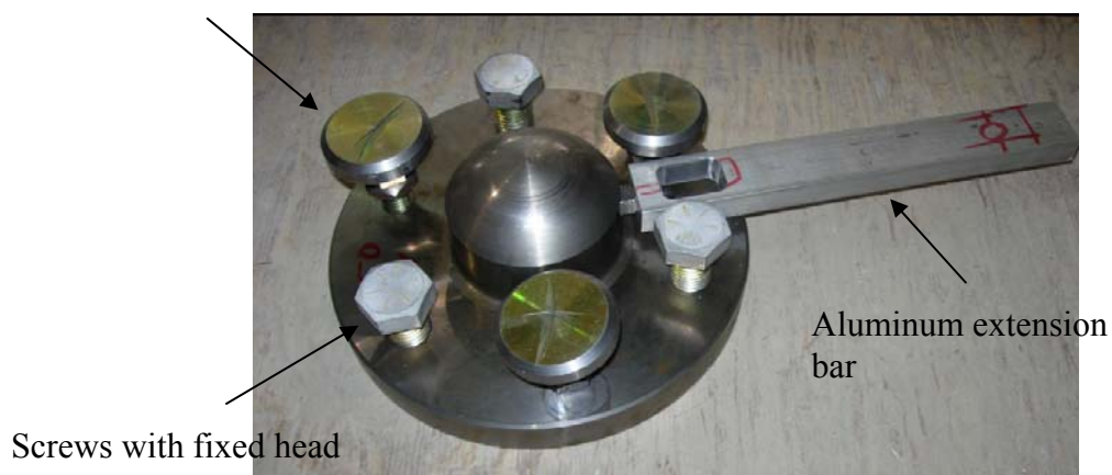
Figure 3.7: Swivel head with additional rigid screws and bar for LVDT
