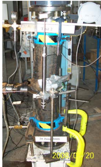
Figure 3.26: LVDTs location after test 1
