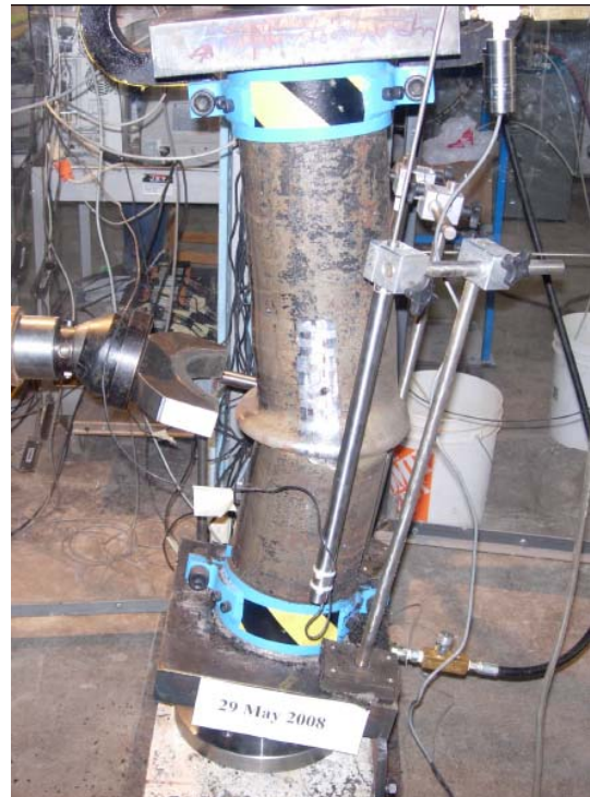
Figure 3.35: Application of the lateral load
