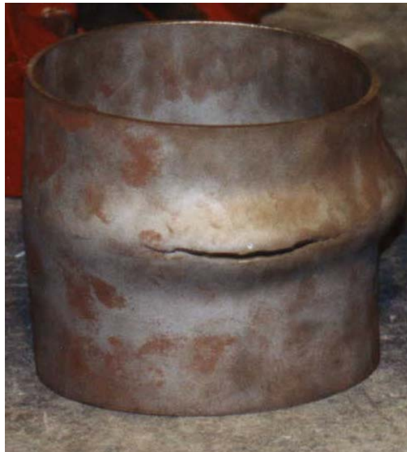
Figure 2.14: Fractured line pipe specimen of Wascana Energy Inc. (Wascana Energy Inc.)
