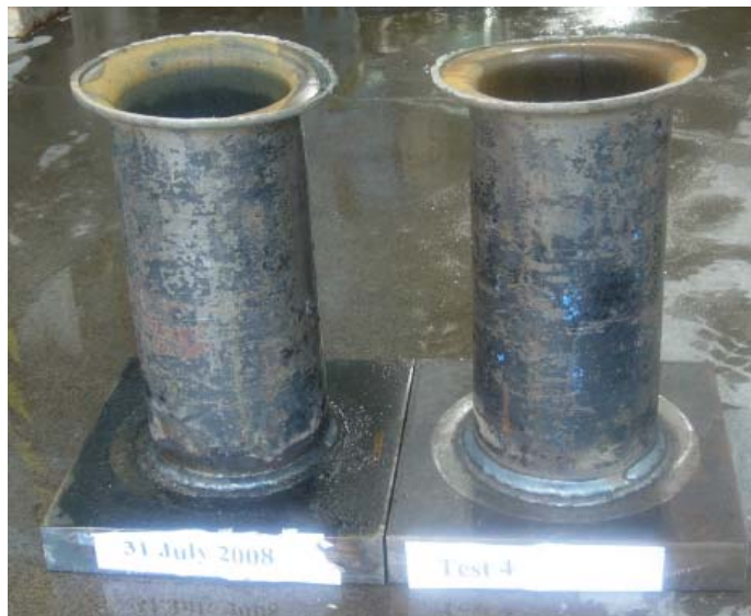
Figure 4.20: Specimen 4 split into two pieces after pressure test
