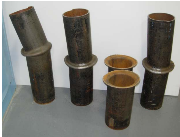
Figure 4.28: Family photograph of specimens 1, 3, 4 and 7 after pressurizing shown from left to right
