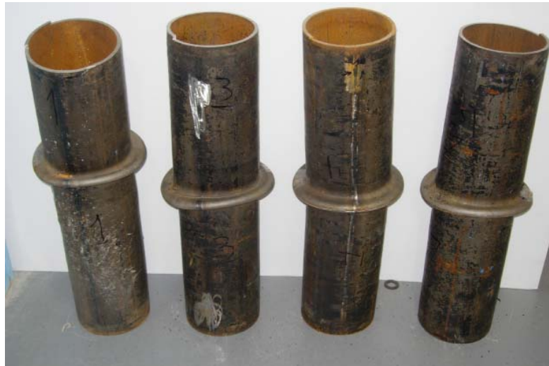
Figure 4.29: Family photograph of specimens 1, 3, 4 and 7 (tension face) shown from left to right
