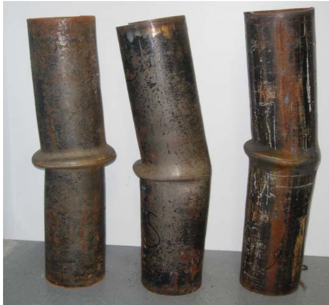
Figure A.17: Family photograph of specimens 2, 5 and 6 before pressurizing
