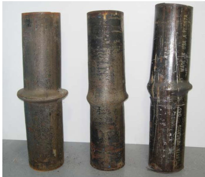
Figure A.20: Family photograph of specimens 2, 5 and 6 (compression face)
