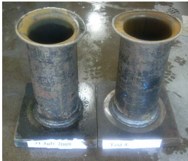
Figure 3.43: Specimen 4 after pressure test
