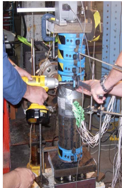
Figure 3.34: Removing the confining collars after starting the wrinkle
