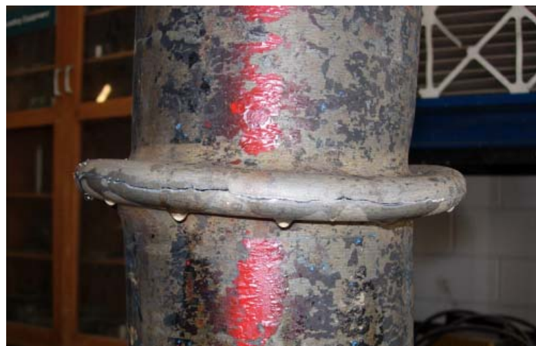
Figure 3.46: Specimen 7 after pressure test
