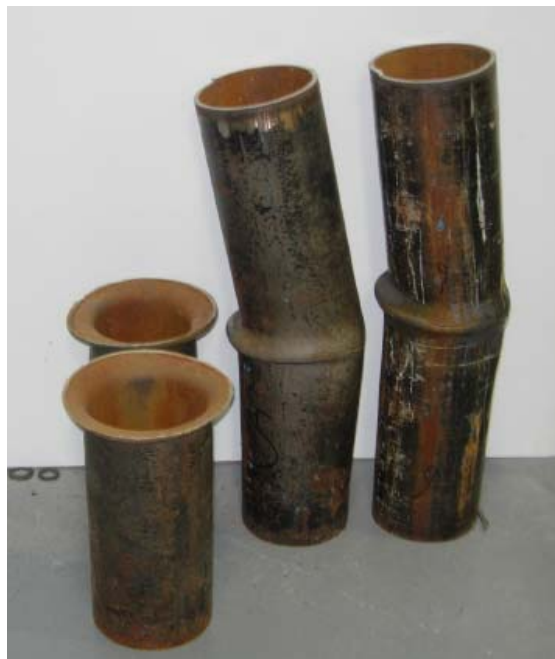
Figure A.18: Family photograph of specimens 2, 5 and 6 after pressurizing
