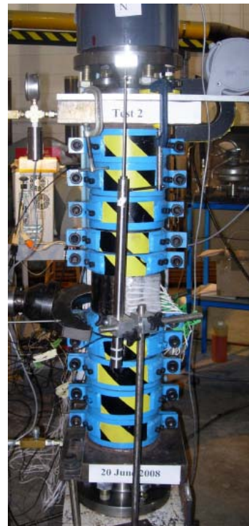
Figure 3.33: Specimen setup and axi-symmetric axial jack loading
