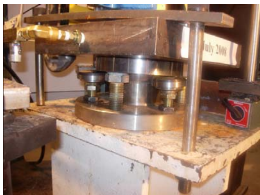
Figure 3.10: Bottom Swivel head loaded after 2° rotation
