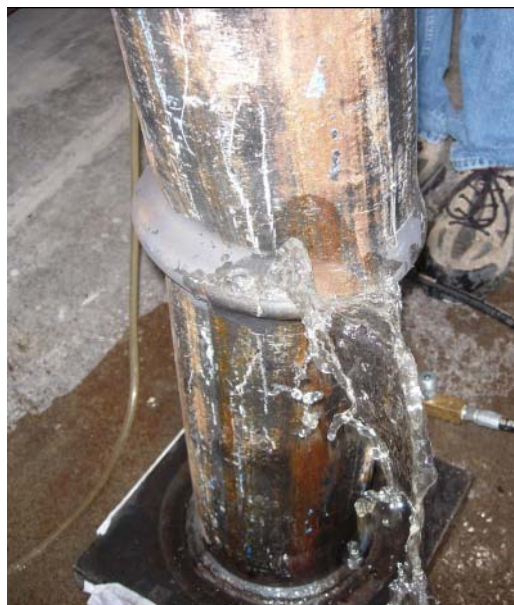
Figure A.16: Specimen 6 after pressure test
