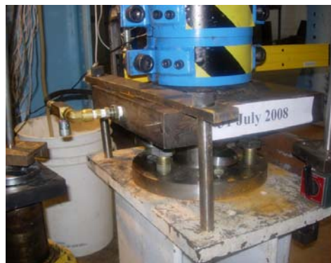
Figure 3.9: Bracing of bottom end plate
