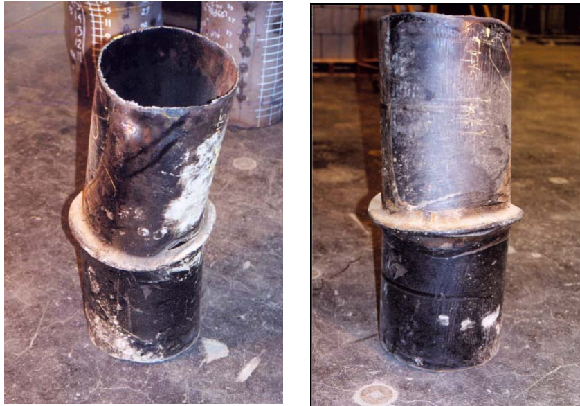
Figure 1.1: Deformed shape of field pipe
