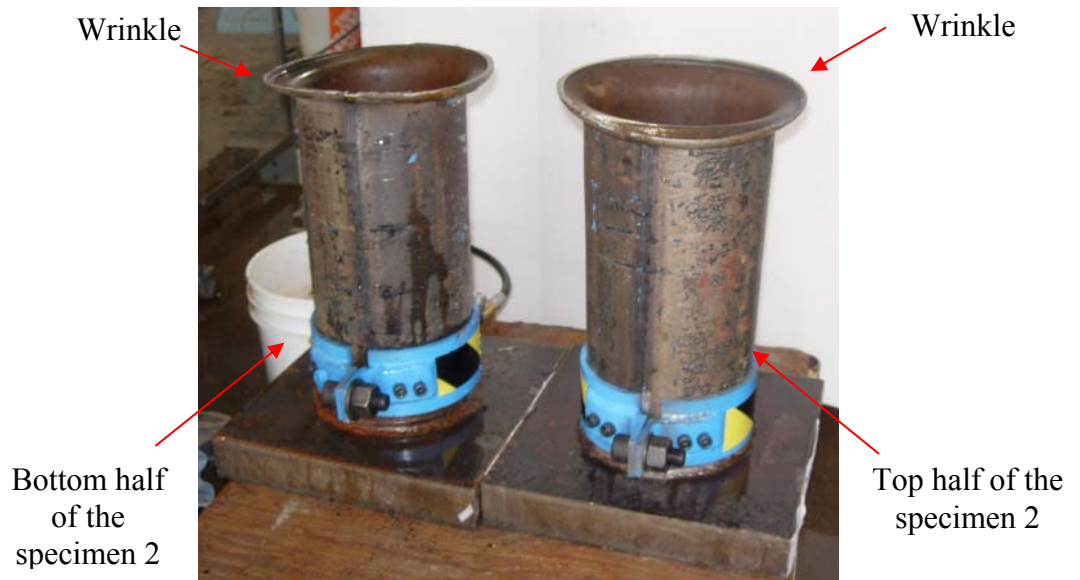
Figure A.4: Specimen 2 split into two pieces after pressure test
