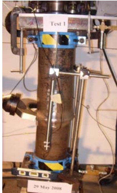
Figure 3.25: Vertical LVDT during 3 rd loading step
