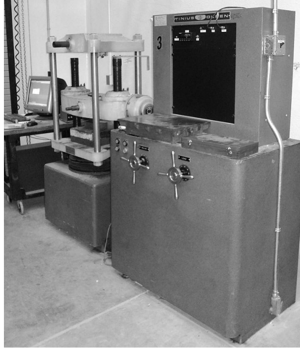
Figure 5.3. 1 Tinius Olsen® tensile/compressive equipment setup
