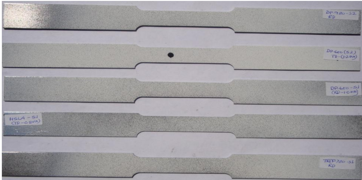
Figure 4.4 Painted tensile test specimens for different grade of sheets with black speckle pattern
