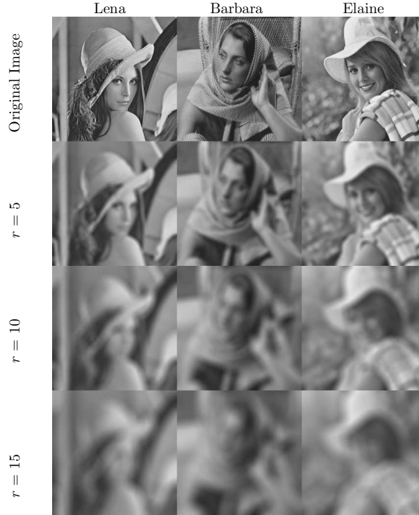
Figure 2.5: Images of Lena, Barbara, and Elaine in their original shape and blurred with disk filters of different radii.
