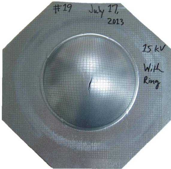
Figure 4-25: Splitting in biaxial DP600 specimens.
