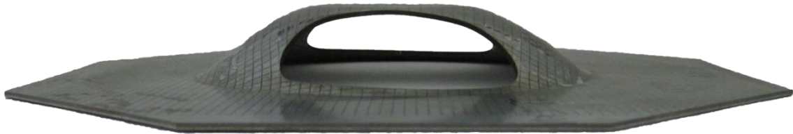
Figure 4-43: Side profile of a mini-die forming specimen with the die lower than the free forming height.
