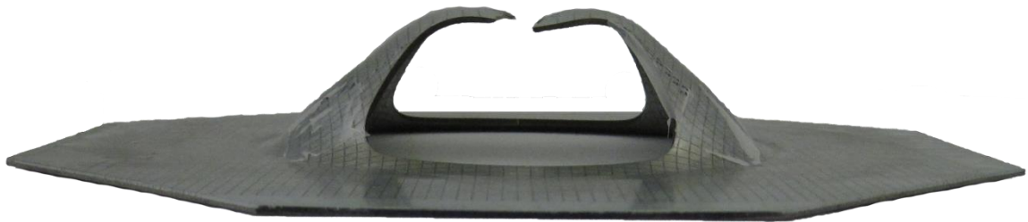
Figure 4-46: Side profile of a mini-die forming specimen with the die higher than the free forming height.
