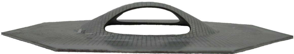
Figure 4-40: Side view of a safe EHFF specimen.
