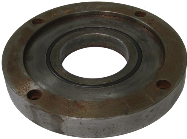
Figure 3-5: The chamber ring that was added to the new chamber to increase the volume.
