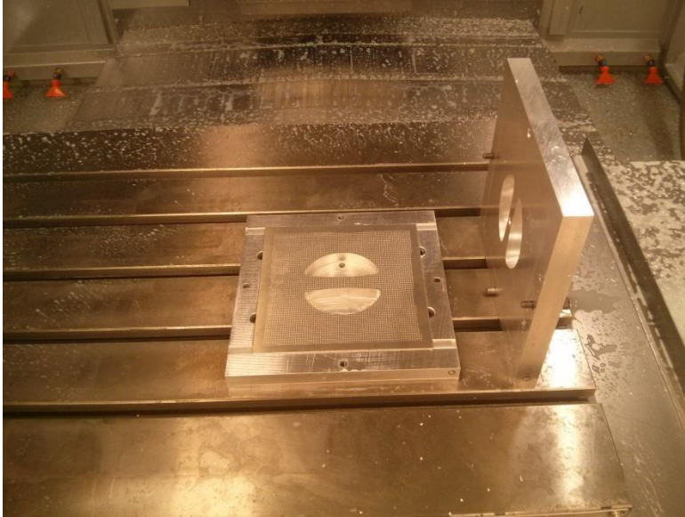
Figure 3-14: A uniaxial specimen in the machining fixture on the bed of the CNC mill.
