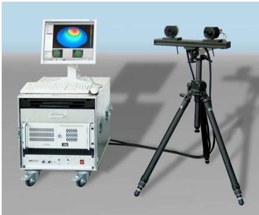
Figure 2.9: the ARAMIS system of the GOM Company
