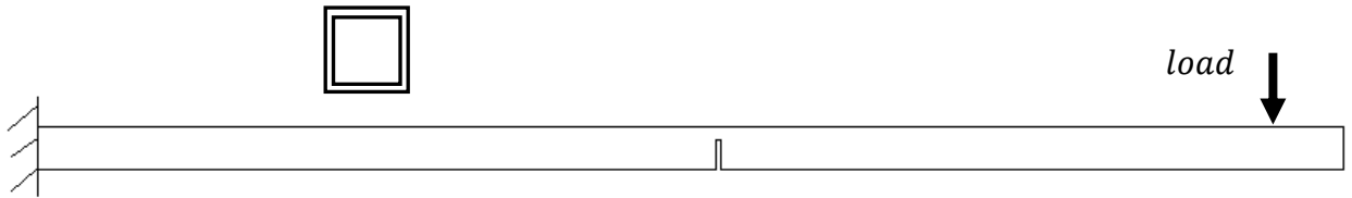
Figure 3.10: Uniform cantilever beam with a saw-cut damage
