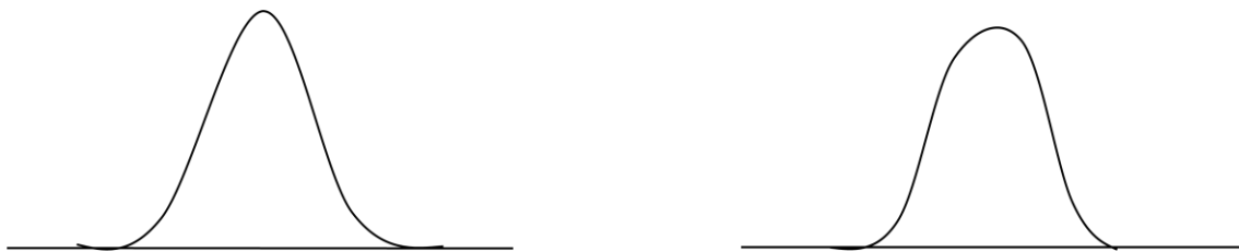
Figure 2.8: Typical design response(s) for low pass filters used for resolution enhancement.
