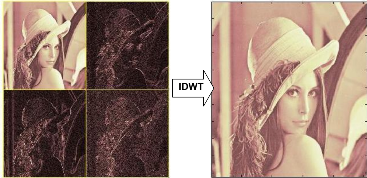
Figure 5.2: The prediction of coefficients for wavelet based super resolution
