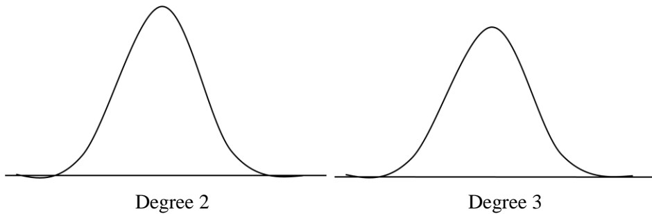
Figure 2.7: The B-splines functions for degrees 0...3
