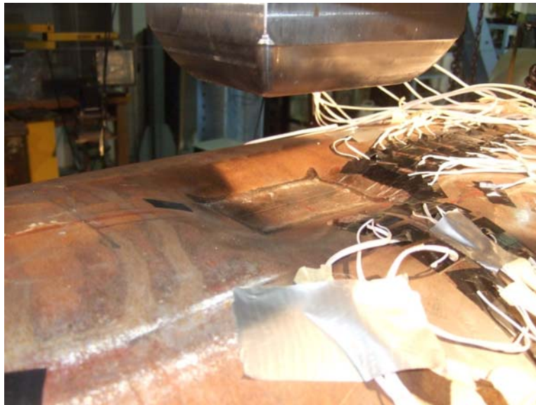
Figure 4.8: Photograph of the dent in specimen LRP40D4
