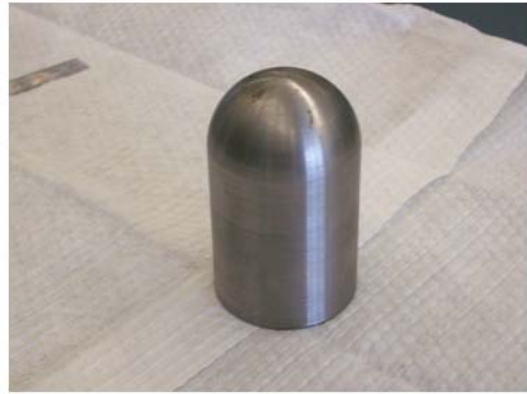
(b) Spherical indenter
