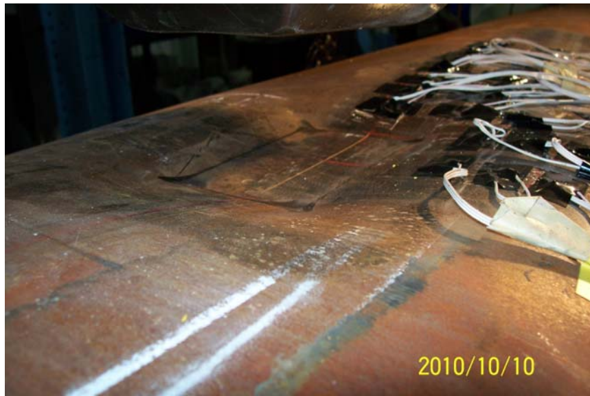
Figure 4.4: Photograph of the dent in specimen LRP20D4
