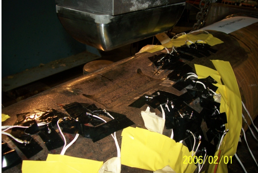
Figure 7.3(a): Photograph of a dent produced by rectangular indenter
