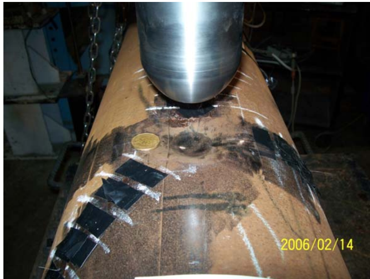
Figure 4.30: Photograph of the dent in specimen SDP20D8
