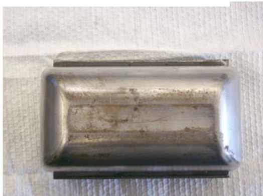
(c) Rectangular indenter for small pipe
