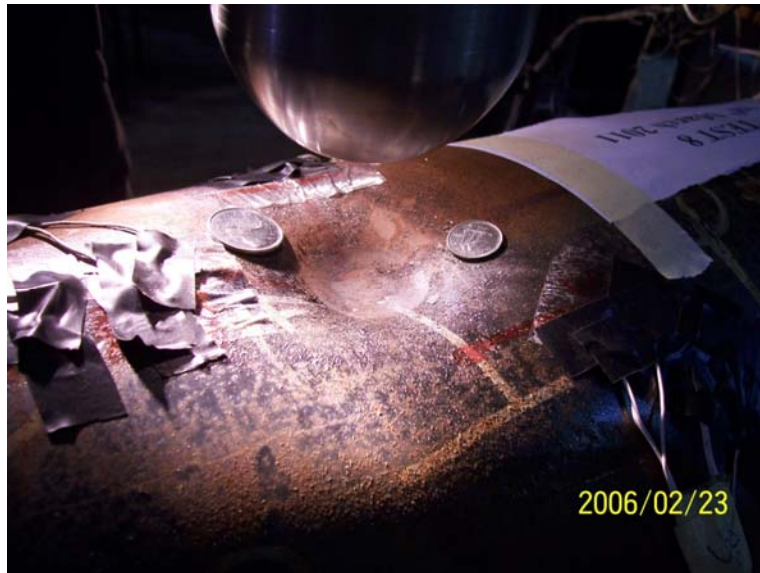
Figure 4.26: Photograph of the dent in specimen SDP0D8
