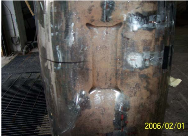
Figure 4.23: Photograph of the dent in specimen SRP20D12
