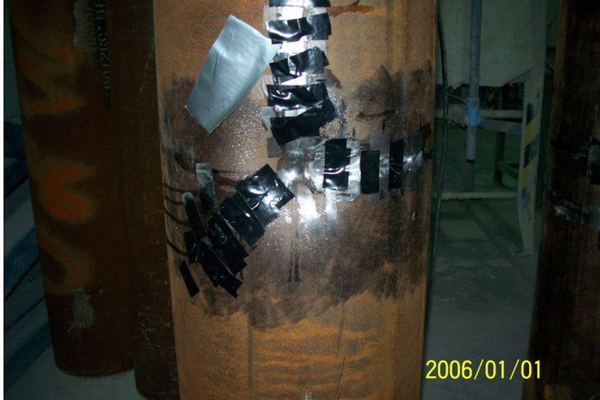
Figure 7.2(a): Photograph of a dent created by a spherical indenter
