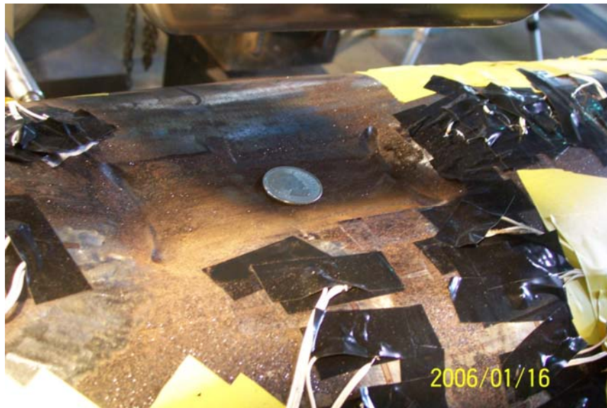
Figure 4.16: Photograph of the dent in specimen SRP20D10
