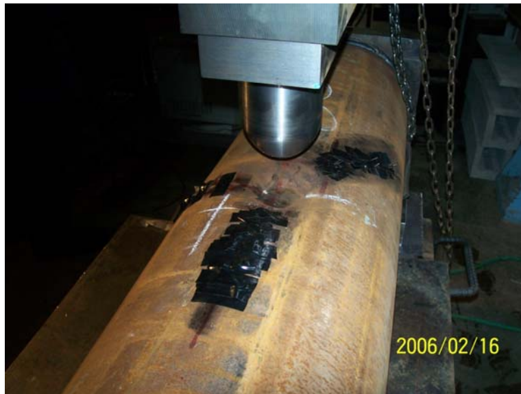
Figure 4.34: Photograph of the dent in specimen SDP40D8
