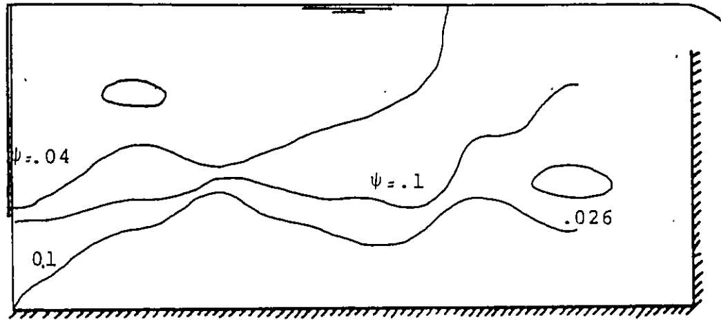
Fig. 5.25 Distribution of (r.m.s.) values for Flow Characteristic ( L = 40 cm, G = 3 cm, \alpha = 61.74 cm 3 /sec/cm).
