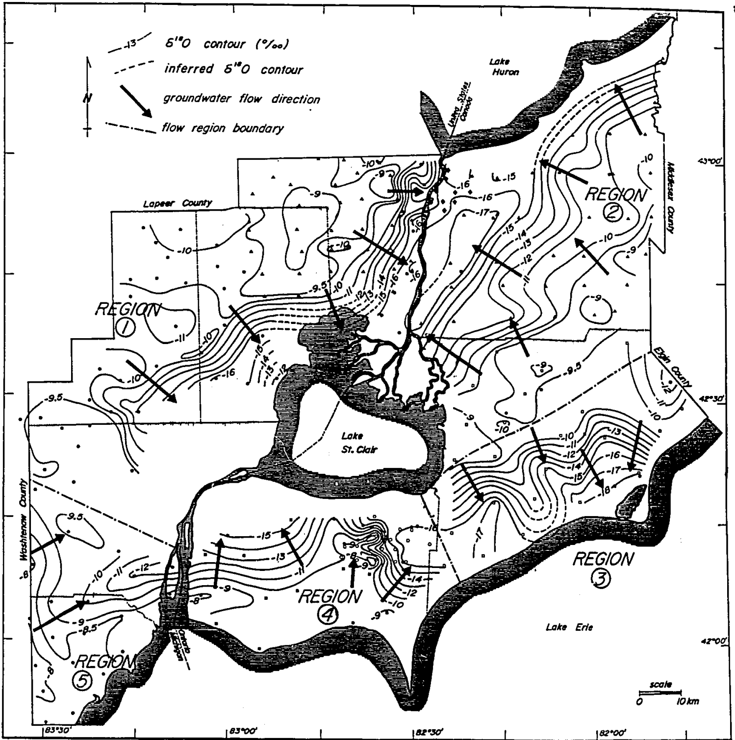
Figure 14 Contour map of oxygen-18 in the freshwater aquifer.
