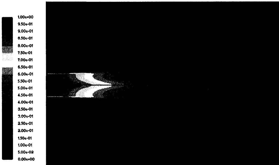
Figure 4.7: Contour of Water Phase Volume Fraction in the Jet (within x/D=10 )
