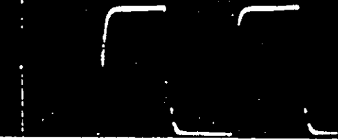
1. SQUARE WAVE, 50 NSEC RISE TIME 1 \mu SEC/DIV HORIZONTAL
